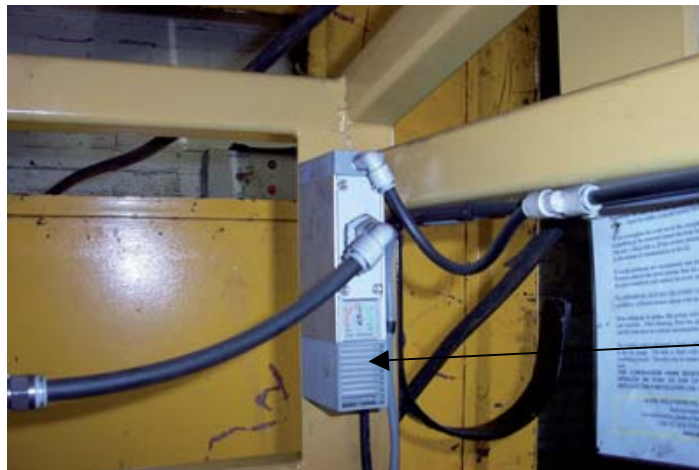
Vacuum generator should not emit vapour
