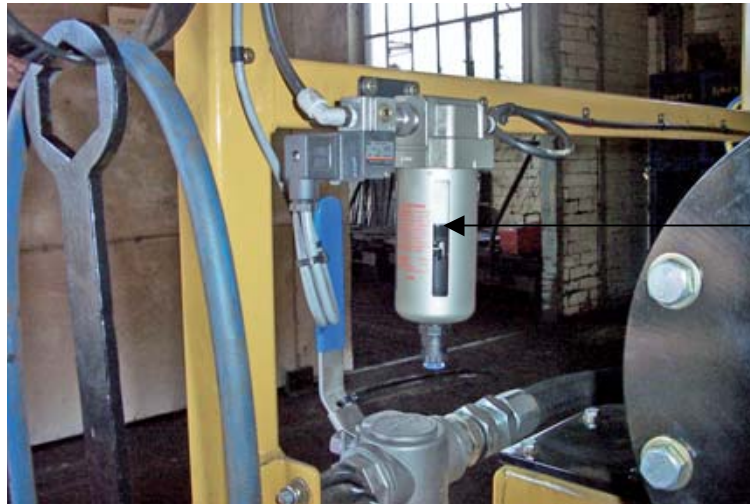
Supply Air filter & water trap
